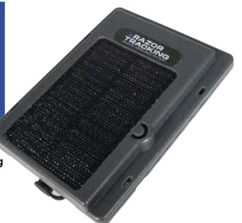
The Solar Hybrid Tracking Device from Razor Tracking is one of the most versatile trackers in the product lineup. It can be used as a real-time tracker: pinging every 30 seconds with power and motion or as an asset tracker pinging 2 times a day. The Solar Hybrid has a rechargeable battery, power harness, and internal antenna. It's ideal for trailers, pull-behinds, NH3 bars, and nurse trailers.
